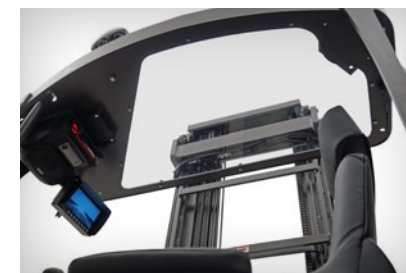
Optional transparent overhead guard roof
