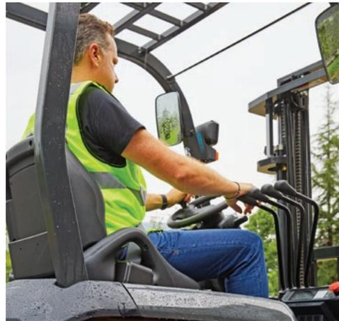
From the spacious operator compartment, with its ergonomically arranged controls, the driver enjoys a great all-round view and a smooth driving experience. Refinements include a high-stability design, pitching control, automatic torque increase and soft mast landing.
