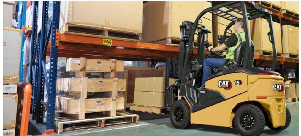
Manoeuvring is fast, precise and safe, thanks to the latest electric hydraulic power steering. Various safety systems – standard and optional – are available to adjust travel, lift and tilt speeds automatically according to the truck's activities at any moment.
