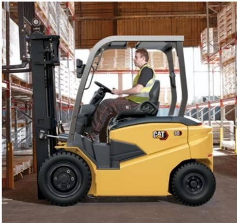
A wide range of capacities is offered, covering everything from light and medium warehouse duties to outdoor tasks. For the heaviest applications, 72 V 3.0 and 3.5 tonne capacity models are available.
