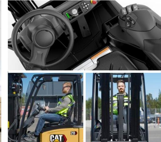
360° steering option gives greater agility in turning. This allows the truck to turn and move in the opposite direction (180°) without stopping, and avoids destabilising the load (3 wheel model).
