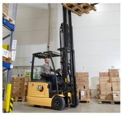
Load-sensing hydraulic system automatically adjusts to the weight being handled, to maintain precise control. Passive sway control keeps the automatic parking brake open so mast sway energy is absorbed by the mass of the whole truck. All masts and low-friction side-shift minimise sway, twisting and noise.
