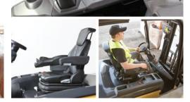
The spacious, high-comfort cabin and its equipment are ergonomically designed to allow strain-free operation with minimal need for the driver to move. Features include a flat, unobstructed floor, adjustable seat and steering wheel, pedals at optimum angles and, to maximise the view, a specially inclined dashboard and counterweight.
