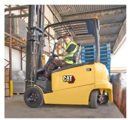
Another great advance over its competitors is the next-generation dual drive 4 wheel steering system, which makes the truck much more manoeuvrable. With +100° rear axle rotation and curve control, turns are tight and smooth. When reversing, side turns can be made immediately without pushing back. Uniquely, the truck can actually be steered using the front axle. As well as giving improved agility and grip, the system reduces tyre wear and stress on the rear axle.
