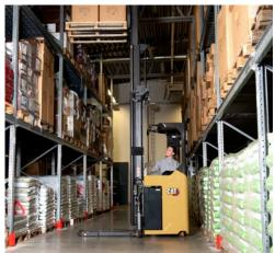
More compact and manoeuvrable than a platform stacker or reach truck, it allows narrowing of your aisles. Meanwhile, its advanced hydraulic, telescoping, drive, steering and stability systems make every operation faster and smoother. The result: better space utilisation and higher handling-cycle work rates.
