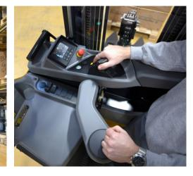
Ergonomic controls give further comfort, job satisfaction and productivity – and avoid stress, strain and fatigue. They include a fully adjustable (up/down, forward/back) steering console, allowing the perfect driver position, and armrestmounted features for simultaneous control of drive and hydraulic functions.
