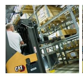
Although specialised for double-deep racking systems, the truck has many other uses. Like handling long loads or reaching across lorry cargo areas. It can act as a reach truck, a four-point straddle stacker, a pallet truck and an order picker.
