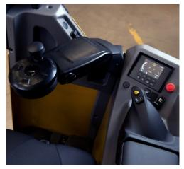
User-friendly controls include fingertip hydraulic levers, with an adjustable armrest, and a positionally adjustable mini steering wheel. The truck's easy and precise manoeuvring and load handling are ideal for a variety of applications and tasks. They include general warehouse work, as well as material flow in factories.
