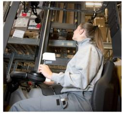
The driver is comfortably seated in a quiet, low-vibration, ergonomically equipped compartment. Fully contained and protected within the truck's robust structure, he or she can work quickly and confidently, hour after hour. Stress, strain and fatigue are minimised. Extra comforts include the option of electrically adjustable floor height.
