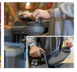
Comfort, job satisfaction and productivity are further enhanced by ergonomic controls which minimise stress, strain and fatigue. These include a fully adjustable (up/down, forward/back) steering console, allowing the perfect driver position, and armrest-mounted features for simultaneous control of drive and hydraulic functions.
