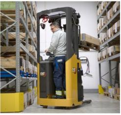
Stand-in stackers enable you to use your valuable warehouse space more fully by making aisles narrower and racking higher. Fulfilling multiple roles, including order picking, they offer similar lifting capabilities to many reach trucks but at lower prices and in tighter spaces.
