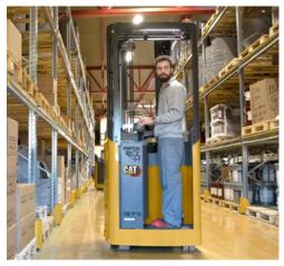
Contained and protected within the truck's robust structure, operators work quickly and confidently – with lower accident and damage risk – thanks to automated speed and stability aids. The operator compartment is vibration-free, comfortable, quiet and very easy to enter and exit.
