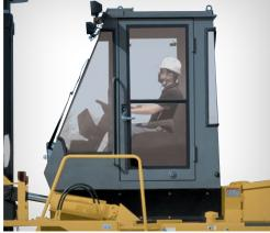
The spacious driver compartment gives clear all-round views. From an adjustable, swivelling, full-suspension seat, ergonomically arranged, loweffort controls are easy to reach. Noise and vibration are minimised by shock-absorbing features. A floating weatherproof cabin and other highcomfort features are optionally available.
