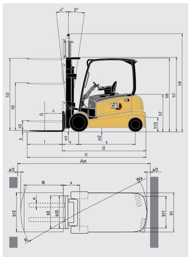
Ast = Working aisle width with load
