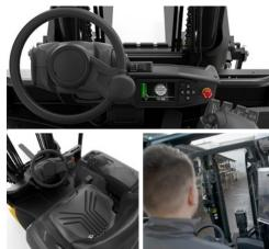
The spacious, high-comfort cabin and its equipment are ergonomically designed to allow strain-free operation with minimal need for the driver to move. Features include a flat, unobstructed floor, adjustable seat and steering wheel, pedals at optimum angles and, to maximise the view, a specially inclined dashboard and counterweight.
