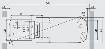
Ast = Working aisle width with load
