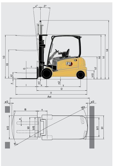
Ast = Working aisle width with load
