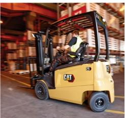
Dynamic aids like *RDS*, *OmniTurn* all-wheel steering and intelligent curve control create a remarkably agile driving experience. When extra acceleration or climbing torque are needed, *PowerBurst* kicks in to give you a boost. Electric differential locking gives additional confidence in slippery conditions.
