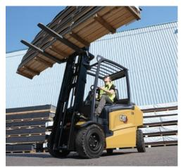
Materials handling is smoother, faster, safer and more precise, thanks to *SmoothFlow* and other hydraulic technologies which optimise mast and fork movements according to load weights and lift heights. Light yet responsive fingertip levers or joysticks give effortless control.
