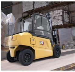
Their exceptional agility gives drivers the feeling of driving a much smaller truck. Dynamic aids include *OmniTurn* all-wheel steering, RDS (Responsive Drive System) and intelligent curve control. *PowerBurst* adds extra acceleration or climbing torque when needed, while electric differential locking helps in slippery conditions.
