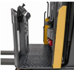
Cushioned, high-grip mat covers wholefloor driver presence sensor. Operation is permitted from any standing position. Walkthrough access is quick and free of tripping hazards, thanks largely to the absence of a traditional 'deadman pedal'.
