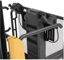
Advanced, user-friendly interface features a right-hand control unit providing excellent anatomical fit, positional adjustment, grip and support, for comfortable and precise operation. Meanwhile, the left hand stays firmly on the Midi steering wheel.
