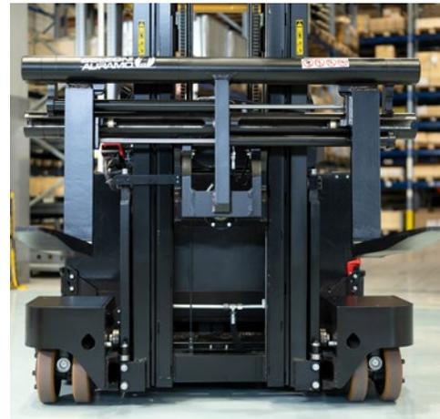
A high-quality fork positioner, with an inbuilt tilt function, provides the wide spread these trucks need. It allows them to carry anything from standard pallets to exceptionally long loads. Pipes, planks and girders, for example. Combined with the all-wheel synchronised steering, it creates an ideal solution for handling such items in narrow aisles.
