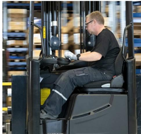
The spacious cabin is furnished with a high-comfort Grammer seat, lined walls and convenient storage features. Advanced fingertip hydraulic controls are embedded into an ergonomic, adjustable armrest. Drivers can operate the adjustable steering wheel from a variety of hand positions.
