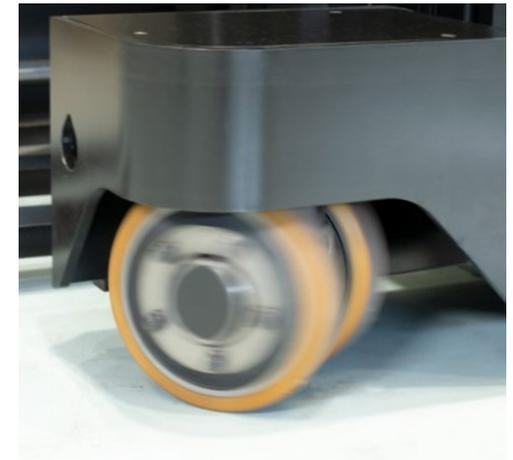
Each load wheel has an independent steering motor, controller and brake system. They can each turn 360° in either direction, for maximum manoeuvrability, speed and precision – whatever the task.
