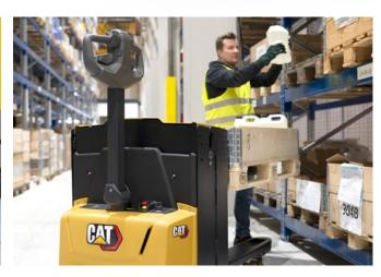
The NPP20N3E is equipped with lifting forks (730 mm height) that offer an ergonomic position for loading and unloading items with minimal physical strain.
