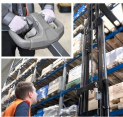
Smooth and precise control characteristics and a comfortable operating position, with a user-friendly tiller arm and excellent visibility through the mast, ensure a satisfying user experience. Height-adjustable castor wheels\* and highstrength masts help to maximise stability.
