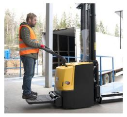
Models with a small fold-down platform are available at 1.0, 1.2\*, 1.4 and 1.6 tonne capacities to take the legwork out of longer distances.
