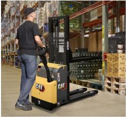
A new compact pedestrian stacker, the 1.2 tonne NSP12N2C, is now available. This powerful but space-saving model is ideal for filling store shelves, stacking, order picking and short internal transport work in, for example, warehouses, supermarkets and production areas.
