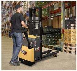
The NPP12N2D pedestrian double pallet handler boosts productivity by carrying two pallets simultaneously (one above the other). It is ideal for loading and unloading on dock levellers, picking and refilling, and transporting loads over short distances in warehouses, supermarkets and production areas.
