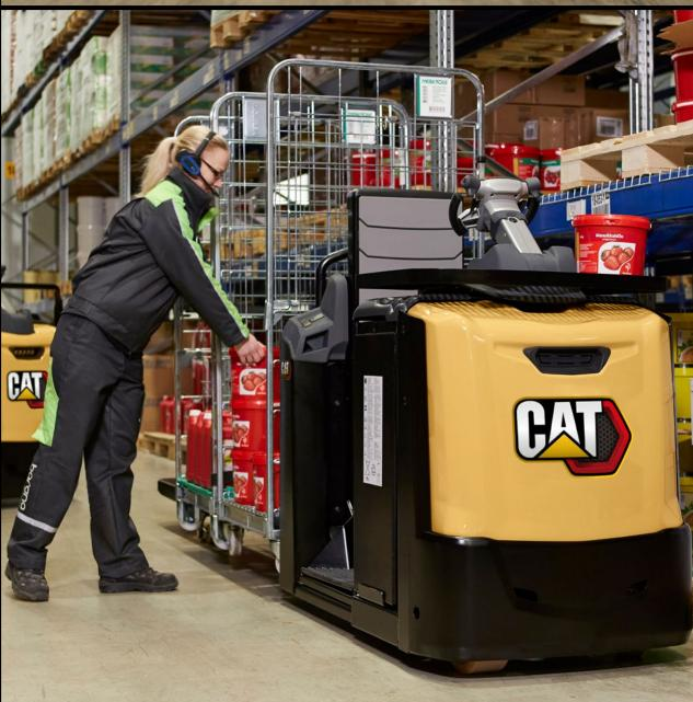
(Pictured clockwise from far left) The **NOH12PH** is designed for high-level picking at heights up to 12.1 m.
