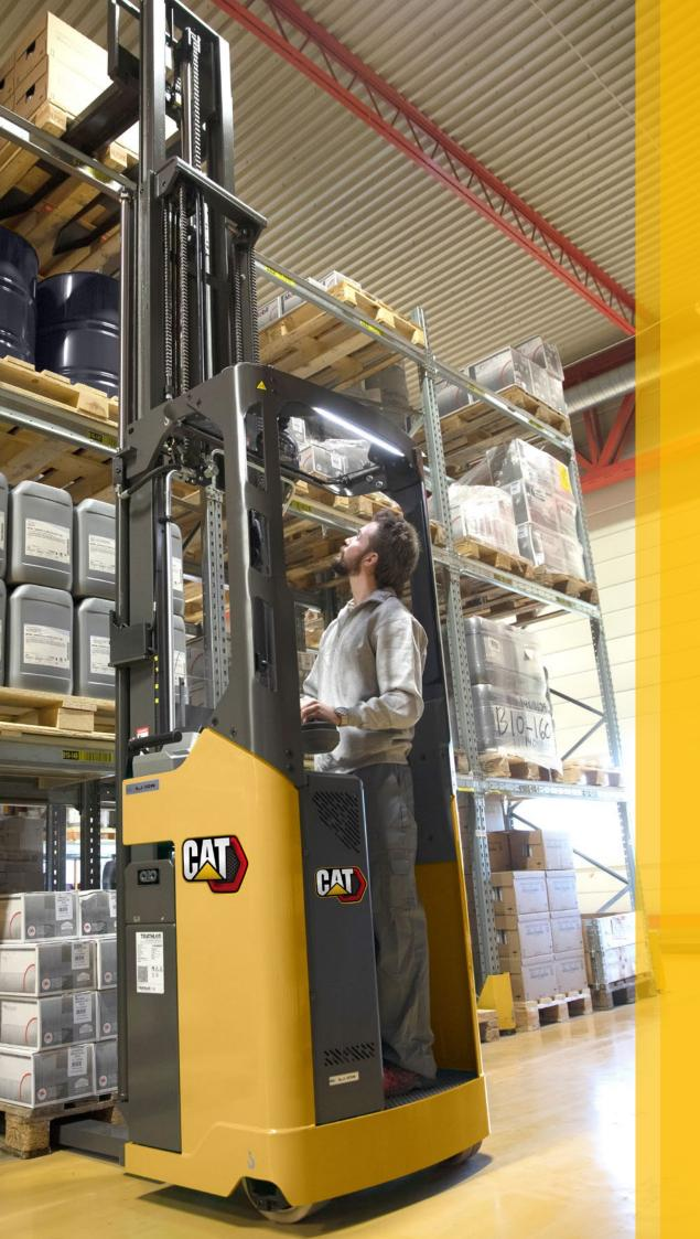
(Pictured far left, from top) The **NSV/NSF12-16N3** range of platform stackers includes initial lift (I) versions that allow ground clearance to be increased for ramp work.
