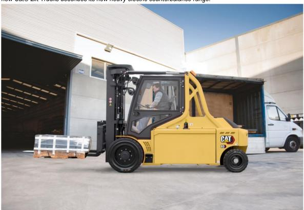
Caption: The spacious operating compartment of the Cat® EP60-120N(H) is rubber-mounted to minimise vibration and noise
