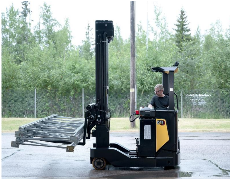
Caption: Here the Cat® NRM25N2 multi-way reach truck used for handling exceptionally long loads in narrow aisles.
